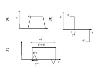
Figure 3.4: Constant voltage pulse (a) and the corresponding electric (b) and magnetic (c) pulses in the bi-filar coil.
