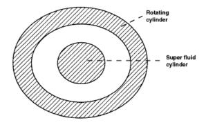
Figure 13.4: Experimental arrangement demonstrating Meissner effect for Super fluids
