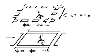
Figure 13.3: The penetration of magnetic field into a super conductor of type I
