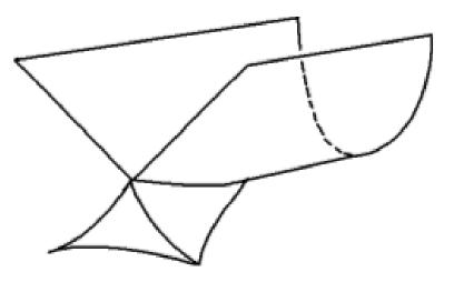
Figure 2.1: The projection of the bifurcation set of the swallowtail catastrophe to the 3-dimensional space of control variables. The potential function has four extrema in the interior of the swallowtail bounded by the triangles, no extrema in the valley above the swallowtail, and 2 extrema elsewhere.
