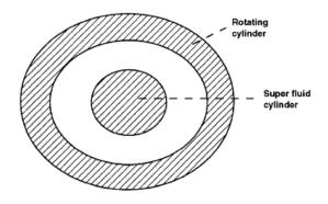
Figure 12.4: Experimental arrangement demonstrating Meissner effect for Super fluids
