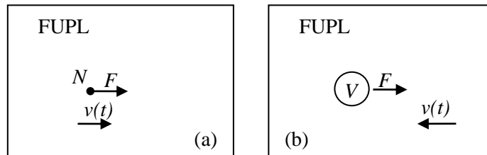
Figure 18 - Sets uholes being moved in a UPL. In (a) N uholes is moving and UPL is stopped; In (b) the volume V associated with the uholes is stopped and the UPL is moving.
