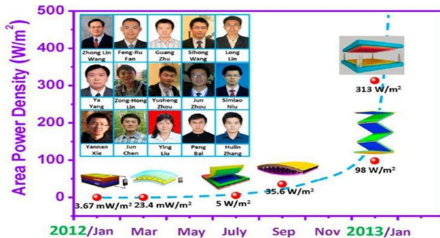
Summary on the progress made in the output power density of a TENG within 12 months. The insets are the people in Wang's group who have made important contributions to the discovery and development of TENG.
