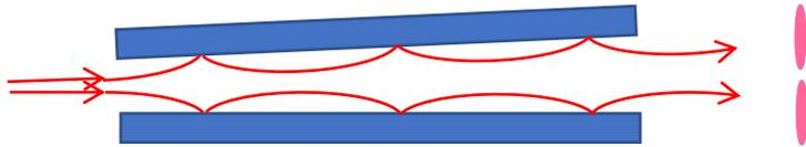
Fig. 15.4. Top view of the plates. Parts of the beam slide along the plates due to the presence of a denser boundary layer near each plate.
