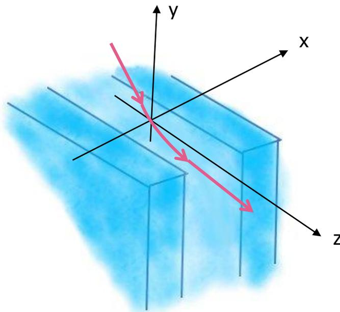
Fig. 15.1. The laser beam enters from above into the gap between the plates and is refracted in their merged boundary layer. This layer is invisible; however, for clarity, it is depicted by a fog in this image, lighter between the plates and darker at the edges of the plates.
