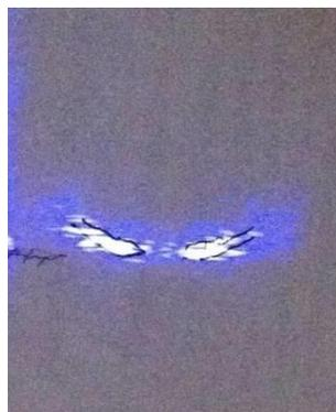
Fig. 15.3. Screen image. The beam width is greater than the gap width; therefore, one can see the traces of rays that have passed at different distances from the plates.
