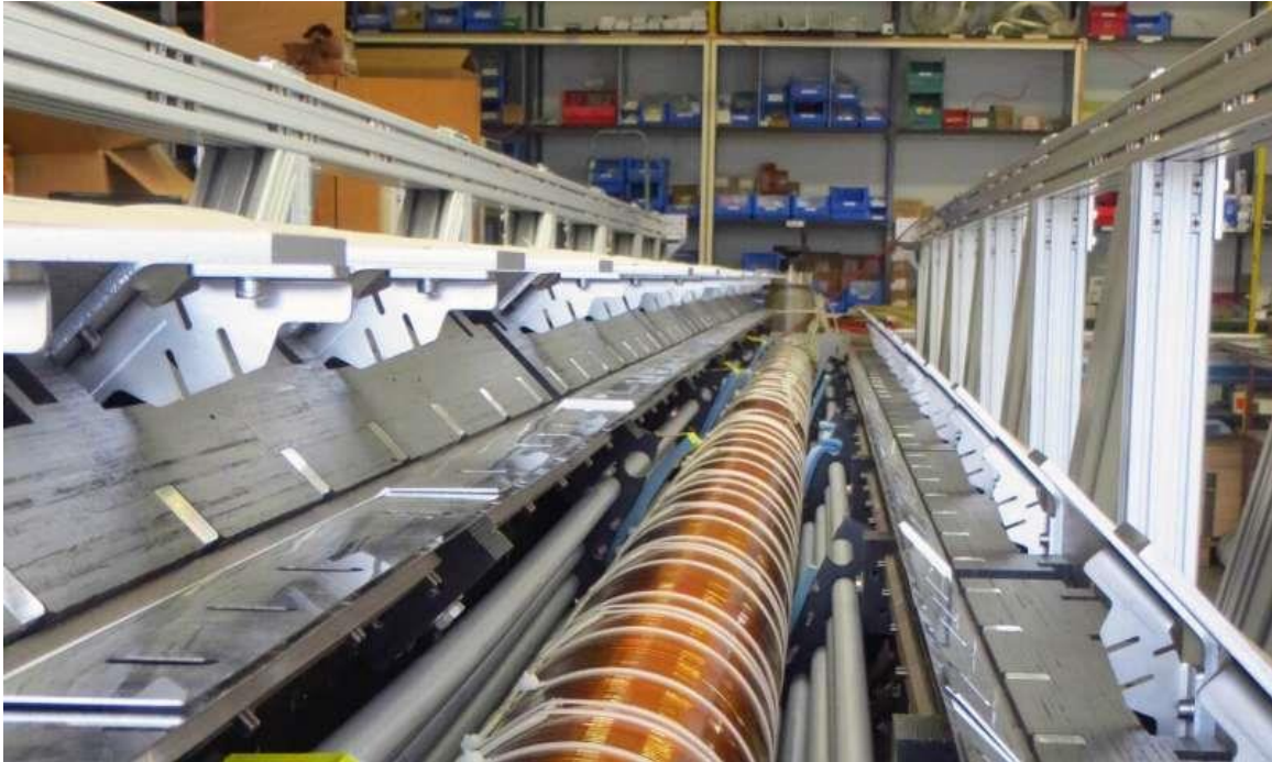
The vacuum chamber for the atomic fountain with magnetic shield. Credit: Leibniz University Hannover
