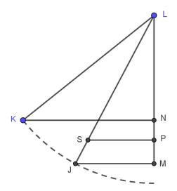
Fig.5. The figure deoicts two inclined plaes, LK and LJ of equal lenghts, their respective heights LN and LM. The times of fall along the planes is equal to the square root of the inverse ratio of their heights.
