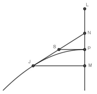
Fig. 6. PJ is the given semi parabola. The vertical through P is its axis. The problem is to locate L, the point from which a particle dropped and reflected at P to move along the horizontal traces the parabola. along the vertical. The composition of these two independent motions gives the parabolic motion.
