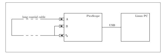
Figure 1: Experimental setup
