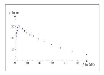
Figure 2: Measured phase error between inputs A and B of the oscilloscope depending on the signal frequency f
