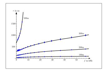
Figure 3: Measured signal delays  $\tau$  between the two channels for sine waves as a function of cable length and signal frequency f
