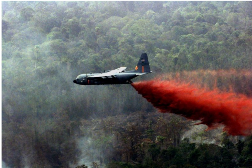
Fig.2. A MAFFS-equipped Air National Guard C-130 Hercules drops fire retardant on wildfires in Southern California
