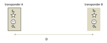
Initially  $S_A$  emits a short light pulse, which will be detected by  $O_B$ , which will trigger  $S_B$  to immediately emit a short light pulse, which will be detected by  $O_A$ , which will trigger  $S_A$  to immediately emit a short light pulse, which will be detected by  $O_B$ , and so on. An electronic counter counts the number of pulses in a given period of time.
