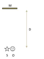
Initially, a short light pulse is emitted by the source S, which will travel to mirror M, and reflected back to the detector O. Upon detecting the light pulse, detector O immediately triggers source S to emit a short light pulse again, which will travel to the mirror, reflected back and detected by O, which triggers source S and so on. A counter counts the number of pulses emitted. If we don't consider the finite time delay between detection and re-emission, the round trip time will be:
