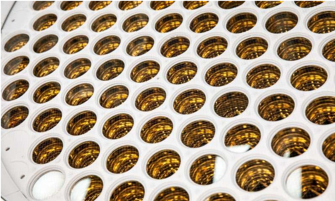
An intricately thin wire grid is visible (click image to view larger size) atop an array of photomultiplier tube. The components are part of the LZ inner detector. Credit: Matt Kapust/SURF
