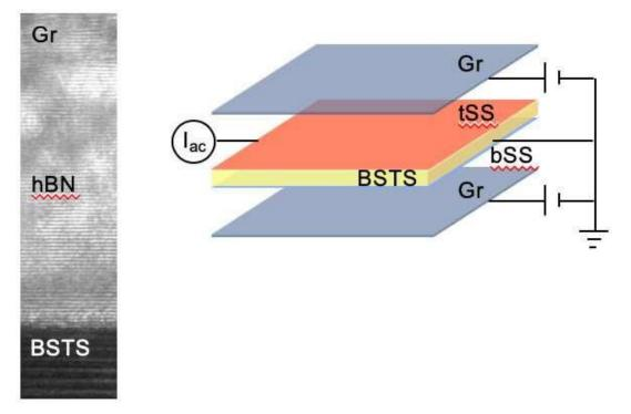
Deshpande and his team created devices using 3-D TIs by stacking five few-atom-thin layers of various materials into sloppy sandwich-like structures. The core of the sandwich is the topological insulator, made from a few quintuple layers of bismuth antimony tellurium selenide (Bi2-xSbxTe3-ySey). Credit: Su Kong Chong
