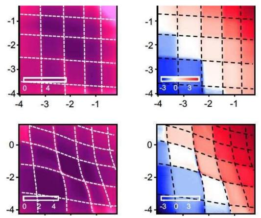
In the presence of the magnetic field, a checkerboard pattern emerged from the metallic surfaces on the 3-D topological insulator devices. These checkerboards allow the researchers to track any distortion on the surface. Thinner insulator layers showed a distorted pattern and at 16 nanometers thickness, the intersection points began to break up. This created a gap that indicated that the surfaces were no longer conductive. Credit: Adapted from Chong et. al. (2019) Physical Review Letters
