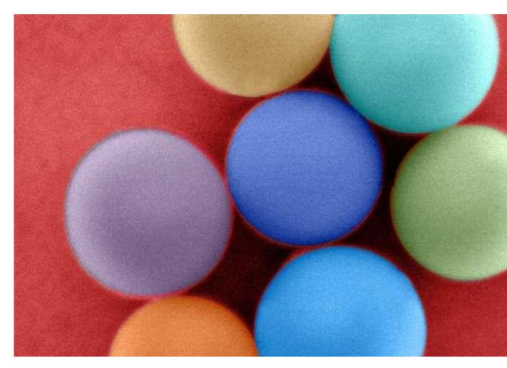
Artist's representation of glass beads of slightly different diameters (denoted by different colors) in the nanoresonator coating. Each bead acts as an optical whispering gallery, or resonator, for a slightly different wavelength of sunlight. Credit: K. Dill, D. Ha/NIST
