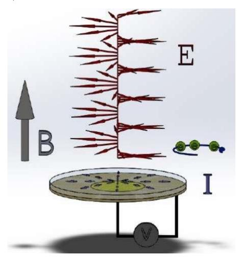
Schematic representation of the experiment. A rotating microwave field (E) is sent through a circular layer of electrons while their electrical current (I) is measured by applying voltage (V). Credit: OIST
