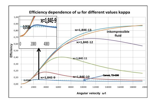
Fig 4: Efficience dependence from  $\omega_1$  for various coefficients of compressibility and for incompressible fluid,  $T_2$ =290
