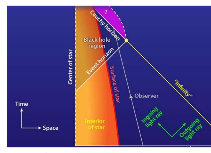
A spacetime diagram of the gravitational collapse of a charged spherical star to form a charged black hole. An observer traveling across the event horizon will eventually encounter the Cauchy horizon, the boundary of the region of spacetime ...more
