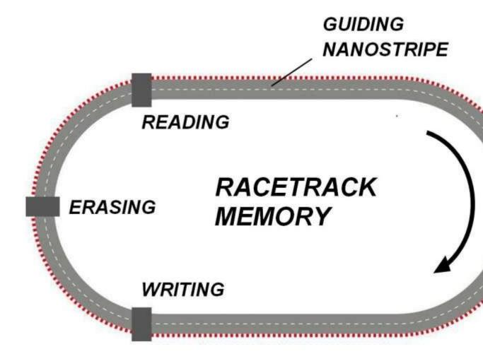
The concept of racetrack memory: magnetic objects move from writing to reading elements. Credit: Forschungszentrum Jülich
