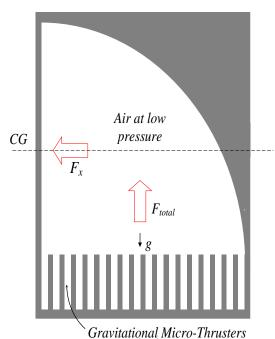
Fig. 4 - The vertical direction  $(-\vec{g})$  of the thrust produced by a plate, with  $N_{\phi}$  gravitational micro-thrusters, can be turned of 90°, in order to produce *horizontal* displacements.
