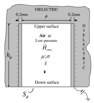
Fig. – 1 Air Cylindrical tube ( $\phi$  diameter;  $h_{\phi}$  height).
