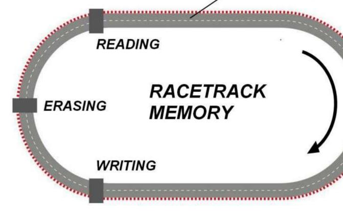
The concept of racetrack memory: magnetic objects move from writing to reading elements. Credit: Forschungszentrum Jülich
