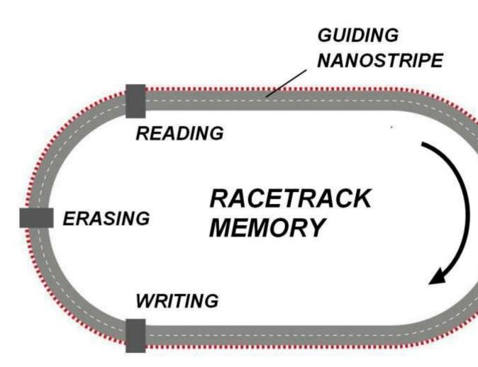
The concept of racetrack memory: magnetic objects move from writing to reading elements. Credit: Forschungszentrum Jülich
