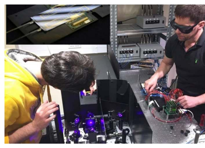
Dr Laing's laboratory where the experiments were performed. Single photons of light are generated using a powerful Ti-Sapphire laser, to pump a series of nonlinear crystals, operated by Ph.D. student and co-author Nicola Maraviglia (left). ...<u>more</u>
