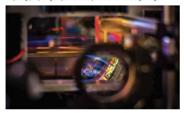
Picture of an optical nanofiber (in red) inside a vacuum chamber. Arrays of individual cold atoms can be trapped around the fiber -about 200 nanometers from the surface- and addressed via the guided light. These "fibered atoms" offer an ...more
