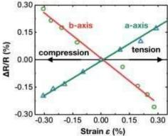
Figure 2. Relative resistance changes of the device along two axes as a function of strain. It shows the relative resistance change of this ReS<sub>2</sub> device along the a- and b-axes, respectively, as a function of the strain. As expected, the a/b-axis showed positive/negative piezoresistance and almost linear change with the strain. Credit: Kanazawa University
