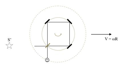
S', which is the apparent point of emission, is at rest, so the speed (group velocity) of light emitted by the source is equal to c in the inertial reference frame in which the device is translating, until it hits the beam splitter. Once the light hits the beam splitter and the mirrors, it
