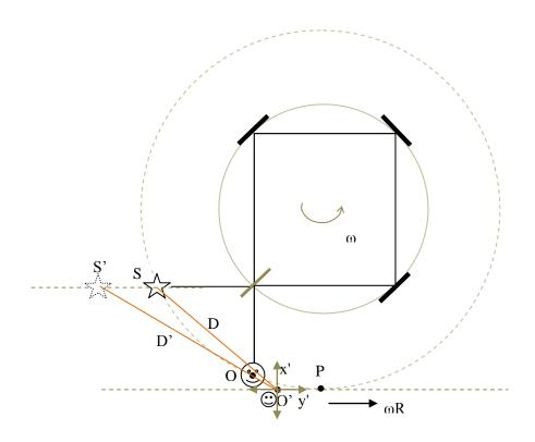
Therefore, we are analyzing the problem in the reference frame of an imaginary inertial observer O' who is moving with velocity of  $\omega R$  to the right. It is as if the Sagnac device is translating to the left (relative to reference frame (x', y')) and rotating at the same time.
