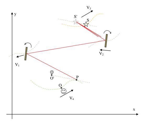
The procedure of analysis is first to define the positions and motions of the mirrors, the beam splitters, the observer/detector and the light source in the absolute reference frame.
