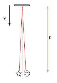
Obviously, for mirror not moving relative to the observer and the light source, the time delay  $t_d$  between emission and detection of light is:
