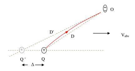
The apparent change in position of a light source depends on the speed of light. In this case, it is *as if* the electrostatic field was 'propagated ' at the speed of light. Actually there is no propagation.
