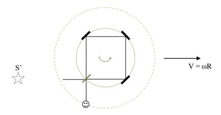
S', which is the apparent point of emission, is at rest, so the speed (group velocity) of light emitted by the source is equal to c in the inertial reference frame in which the device is translating, until it hits the beam splitter. Once the light hits the beam splitter and the mirrors, it
