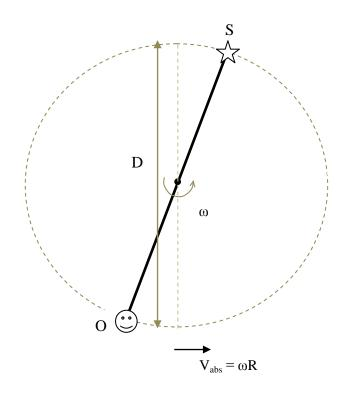
The problem is to determine the path, the path length, the time delay and phase of a photon emitted by the light source and detected by the observer.
