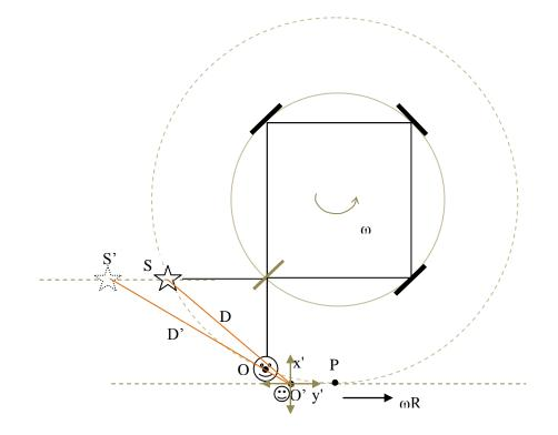
Therefore, we are analyzing the problem in the reference frame of an imaginary inertial observer O' who is moving with velocity of  $\omega R$  to the right. It is as if the Sagnac device is translating to the left (relative to reference frame (x', y')) and rotating at the same time.
