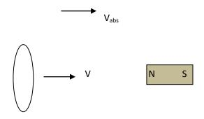
Since the conductor and the magnet are co-moving absolutely, the magnet appears to be closer than its actual/physical distance to the conductor, as seen by the conductor, but the conductor appears farther than its actual distance, as seen by the magnet.
