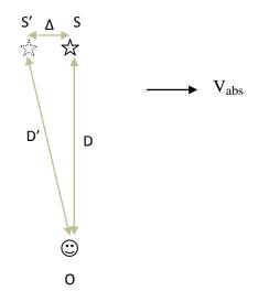
In this case also, the effect of absolute velocity is to create an apparent change in the *position* ( distance and direction ) of the light source relative to the observer.
