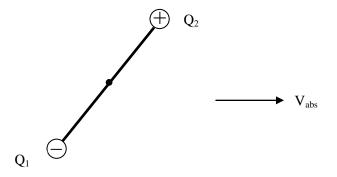
Trouton and Noble reported a null result, that no torque was observed. However, in a recent experiment [9] a positive result was observed and it has been proposed that the original Trouton-Noble experiment gave a null result because the capacitors were put in an electrostatic shield, possibly shielding the capacitors from any absolute motion effect.
