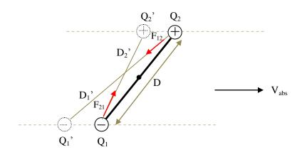
$F_{21}$  is the force of  $Q_2$  on  $Q_1$  and  $F_{12}$  is the force of  $Q_1$  on  $Q_2$ . Although  $F_{21}$  and  $F_{12}$  create opposite torques that will tend to cancel each other, there will be a net torque because the two torques are not exactly equal. This net torque will tend to orient the rod connecting  $Q_1$  and  $Q_2$  perpendicular to the direction of absolute velocity.
