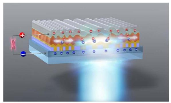
Schematic representation of an organic semiconductor laser diode producing blue laser emission under electrical excitation. Credit: Center for Organic Photonics and Electronics Research, Kyushu University
