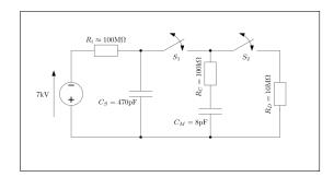
Fig. 7: charging circuit
