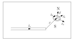
Fig. 3: Small conductor loop as model of a permanent magnet in the vicinity of the wire stub
