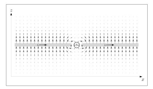
Fig. 4: The force effect of a direct current according to Maxwell onto a permanent magnet with north pole pointing into the drawing plane. The current can be driven by a current source.
