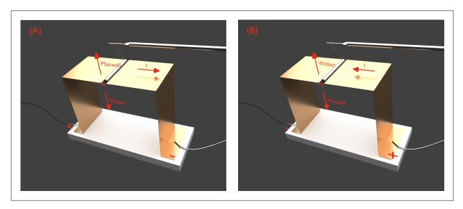
Fig. 6: Experimental setup: capacitor and permanent magnet (north pole directed towards the observer)
