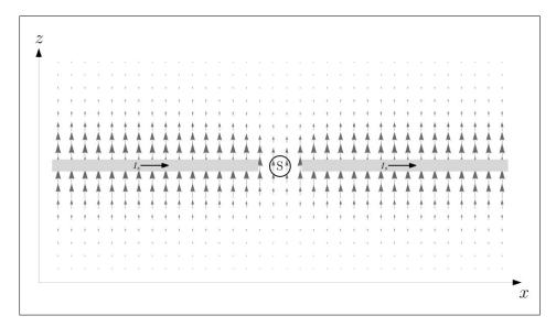
Fig. 5: The force effect of a direct current according to Weber onto a permanent magnet with north pole pointing into the drawing plane. The current can be driven by a current source.
