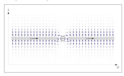
Figure 5: The force effect of a current according to Maxwell onto a permanent magnet with north pole pointing into the drawing plane.
