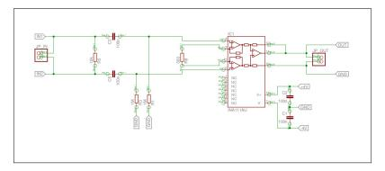
Figure 9: measuring amplifier
