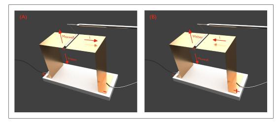
Figure 7: Experimental setup: measuring capacitor and permanent magnet with north pole directed towards the observer
