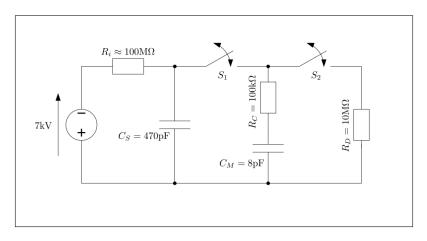
Figure 8: charging circuit
