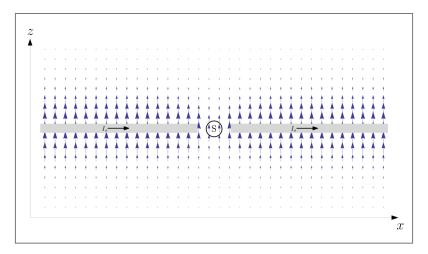
Figure 6: The force effect of a current according to Weber onto a permanent magnet with north pole pointing into the drawing plane.
