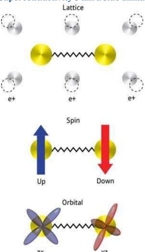
Shimojima and colleagues were surprised to discover that interactions between electron spins do not cause the electrons to form Cooper pairs in the pnictides. Instead, the coupling is mediated by the electron clouds surrounding the atomic cores. Some of these so-called orbitals have the same
