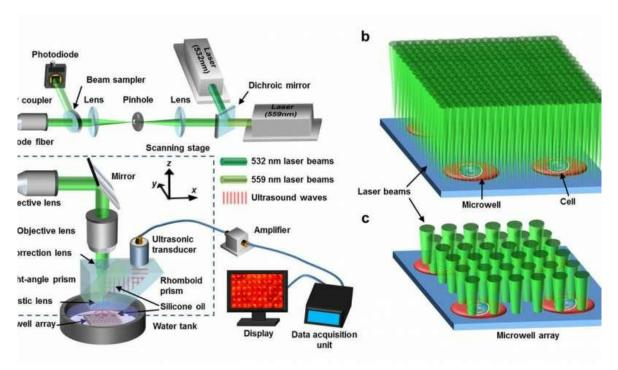
The photoacoustic microscopy apparatus used for imaging the metabolic rates of cancer cells. Credit: Caltech
