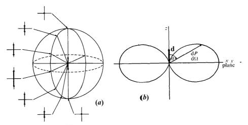
Fig. 1. An electric dipole oscillating parallel to the *z*-axis. (a) Polarization of the electric field seen by looking from different direction [9]. (b) Angular distribution of the radiated energy [1 (67.7)], [2 (9.23)], [3 (2.72]  $dP/d\Omega = \omega^4 d^2 \sin^2 \theta/32\pi^2 \varepsilon_0 c^3$ .
