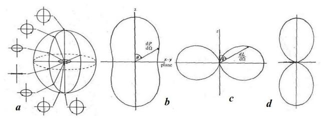
Fig. 2. An electric dipole rotating in the *x*-*y* plane
