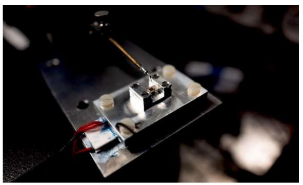
Spin lasers whose oscillation frequency can be mechanically controlled via the mount. Electrical contact can be made via an adjustable needle. Credit: RUB, Kramer
