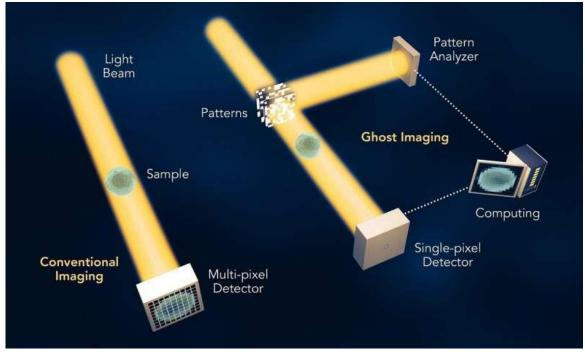
In conventional imaging (left), light falling on an object produces a two-dimensional image on a detector. Ghost imaging (right) constructs an image by analyzing how random patterns of light shining onto the object affect the total amount of light coming off the object. Credit: Greg Stewart/SLAC National Accelerator Laboratory
