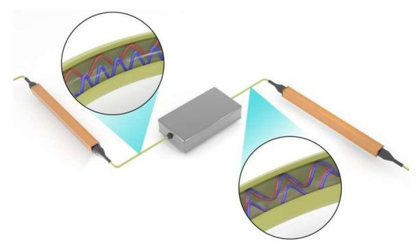
The researchers' innovative experimental setup involved operating on photons contained within a single fiber-optic cable. This provided stability and control for operations producing entangled photons, shown separated at top and intertwined ...more "We were able to extract more
