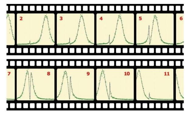
The effect of a single molecule on the cavity's transmission spectrum. The cavity frequency was tuned across the molecular frequency (1-12). When the molecule is on resonance with the cavity (see 7, 8), it blocks completely the transmission ...more
