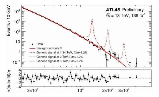
Measured dielectron mass distribution for the data (black points), together with the total background fit result is shown (red continuous line), with various possible Z' signal distributions overlaid (dashed red line). The sub-panel shows ...more
