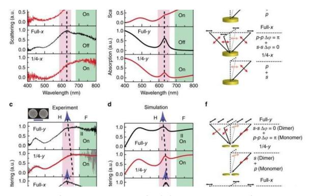
Demonstration of plasmonic switching by dark field (DF) scattering measurement of gold nanodisk monomer and dimer. a Normalized DF scattering spectra of gold nanodisk monomer with a diameter of 200 nm (SEM image) under full and quarter ...more
