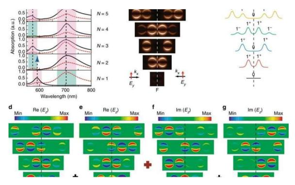
Plasmonic encoding in gold nanodisk chains. a Calculated absorption spectra of gold nanodisk chains consisting of different numbers of nanodisks illuminated by the s-polarized in-plane plan wave coming from right side (dashed line) or both ...more
