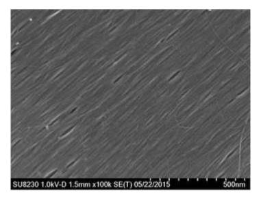
A scanning electron microscope image shows highly aligned and closely packed carbon nanotubes gathered into a film by researchers at Rice. Credit: Kono Laboratory
