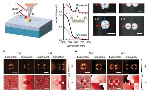
Demonstration of electrical-field distribution rule for the 200 nm gold nanodisk monomer and dimer by s-SNOM. a Schematic of the s-SNOM measurement for s–s and s–p excitation–collection configurations. The wavelength of the excitation laser ...more
