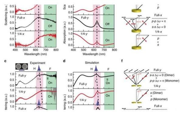
Demonstration of plasmonic switching by dark field (DF) scattering measurement of gold nanodisk monomer and dimer. a Normalized DF scattering spectra of gold nanodisk monomer with a diameter of 200 nm (SEM image) under full and quarter ...<u>more</u>
