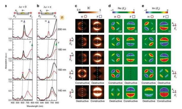
In-plane coherent control of plasmon resonances in gold nanodisk monomers. a, b Calculated normalized absorption spectra of gold nanodisk monomers with a diameter ranging from 140 to 200 nm for s-polarized in-plane plan wave coming from the ...<u>more</u>
