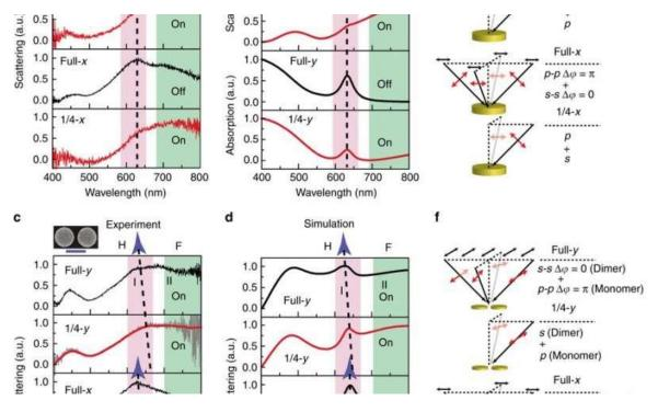
Demonstration of plasmonic switching by dark field (DF) scattering measurement of gold nanodisk monomer and dimer. a Normalized DF scattering spectra of gold nanodisk monomer with a diameter of 200 nm (SEM image) under full and quarter ...<u>more</u>
