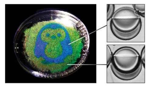
An image of a penguin reflected from oil in water droplets; images of each type of droplet reflecting the blue and green light are shown. The penguin is made by using a light responsive surfactant and photopatterning the droplet shape. Credit: Zarzar laboratory, Penn State
