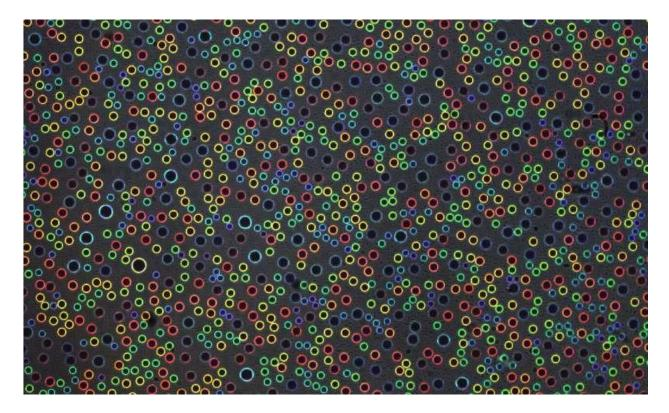
Structural color from clear water droplets. Microscale water droplets condensed onto a clear plastic sheet reflect different bright colors based on their size. Credit: Zarzar laboratory, Penn State
