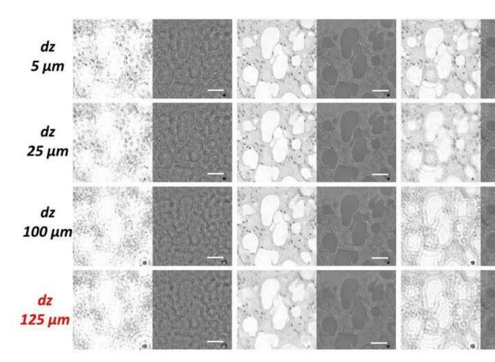
Comparison of HIDEF results against free-space back-propagation (CNN Input) and multi-height phase recovered (MH Phase Recovered) results, as a function of axial defocus distance (dz). Credit: UCLA Ozcan Research Group
