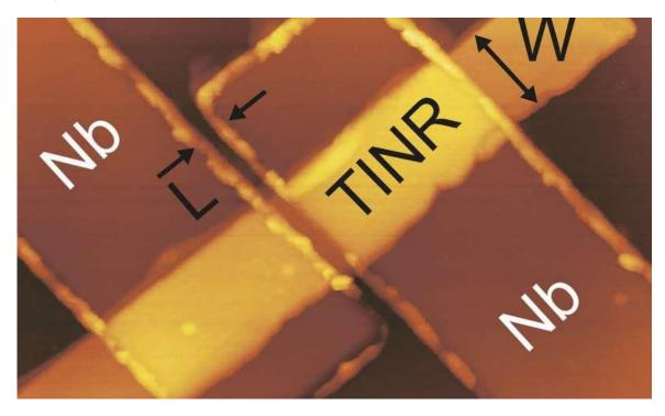
An enhanced supercurrent on the surface of this device's topological insulator could bring special properties that make qubits more resilient. Credit: Purdue University image/Morteza Kayyalha
