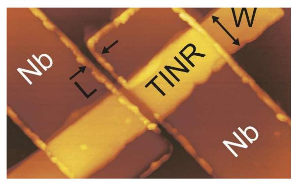
An enhanced supercurrent on the surface of this device's topological insulator could bring special properties that make qubits more resilient. Credit: Purdue University image/Morteza Kayyalha
