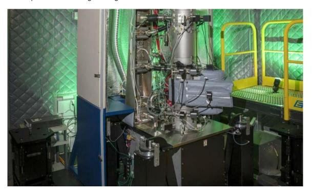
Oak Ridge National Laboratory scientists used a monochromated, aberration-corrected scanning transmission electron microscope, or MAC-STEM, technique that detects the subtle changes in the weight of proteins at the nanoscale--while keeping ...more "Now, we can track isotopic labels directly with the electron microscope, meaning we can do it with a spatial resolution comparable to the actual size of the proteins," Hachtel added.
