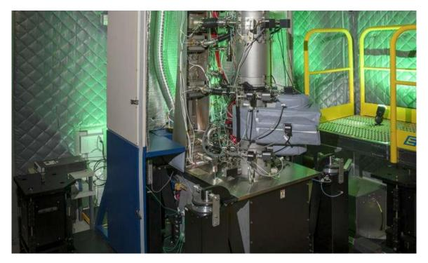
Oak Ridge National Laboratory scientists used a monochromated, aberration-corrected scanning transmission electron microscope, or MAC-STEM, technique that detects the subtle changes in the weight of proteins at the nanoscale--while keeping ...<u>more</u>"Now, we can track isotopic labels
