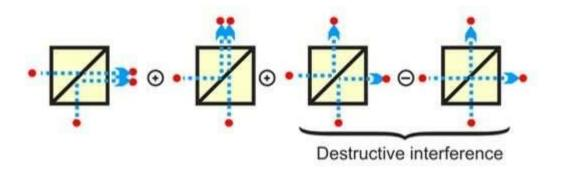
Schematic illustration of the HOM bunching effect of indistinguishable photons in a Beam Splitter. Credit: *Science Advances*, doi: 10.1126/sciadv.aat1451
