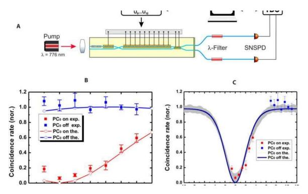
Experimental setup and quantum results. (A) Experimental setup for quantum characterization of the active HOM chip. A tunable narrowband continuous-wave pump laser around 776 nm is coupled into the channel with the PDC source. To avoid ...more
