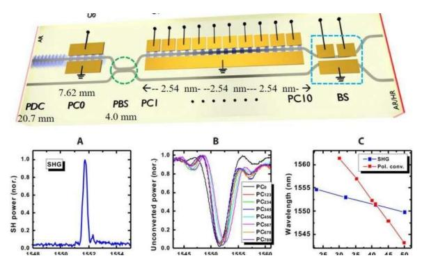
Upper panel: Schematic illustration of the integrated quantum optic chip with monolithic inclusions of a PDC source (20.7 mm), electro-optic PCs (7.62 mm), PBS, highlighted in green (4.0 mm), BS highlighted in blue, and a single element of ...more
