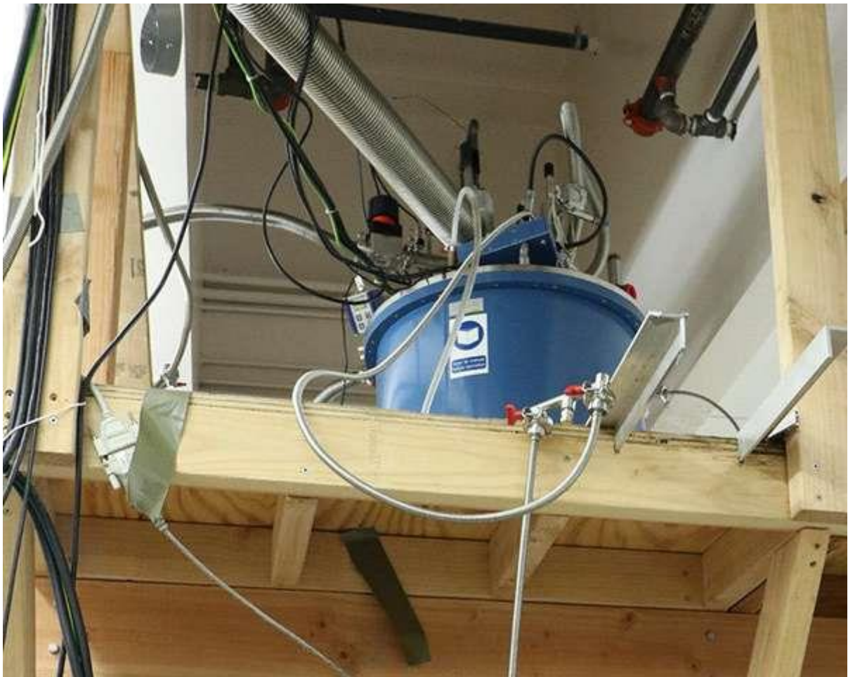
Optical dilution refrigerator for low-temperature experiments at UC San Diego. Credit: Michelle Fredricks
