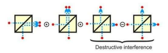
Schematic illustration of the HOM bunching effect of indistinguishable photons in a Beam Splitter. Credit: *Science Advances*, doi: 10.1126/sciadv.aat1451
