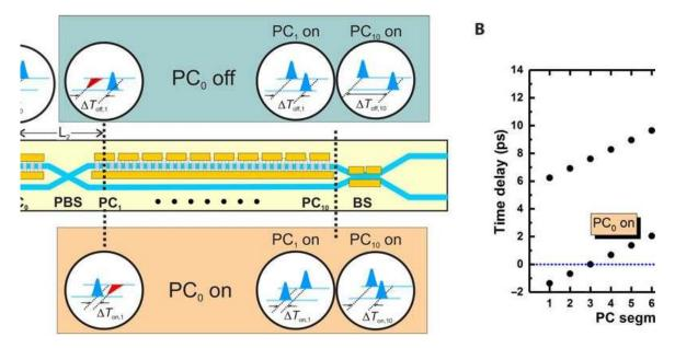
Illustration of the principle of the adjustable BED line. (A) The diagram shows the chip design together with some insets illustrating the temporal relation of the horizontally (red) and vertically (blue) polarized photon wave packets at ...more
