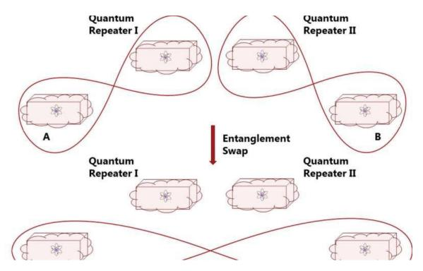
Illustration: When distributing entanglement between sender A and receiver B, the communication line is segmented by inserting quantum repeaters. In this illustration A is entangled with Quantum Repeater I while B is entangled with Quantum ...<u>more</u>
